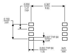
Figure 6. SSOP Footprint (Case 1317 and 1317A)
