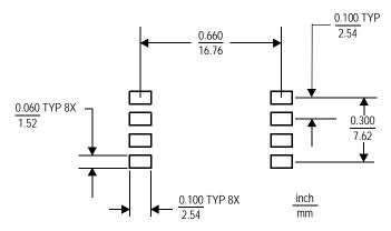
Figure 5. SOP Footprint (Case 482)
