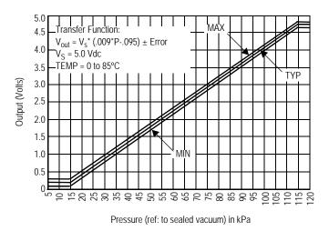
**Figure 4. Output versus Absolute Pressure**
